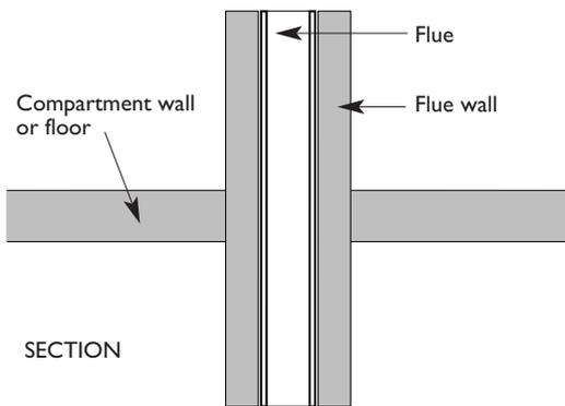
Flue walls should have a fire resistance of at least one half of that required for the compartment wall or floor, and be of non-combustible construction.
