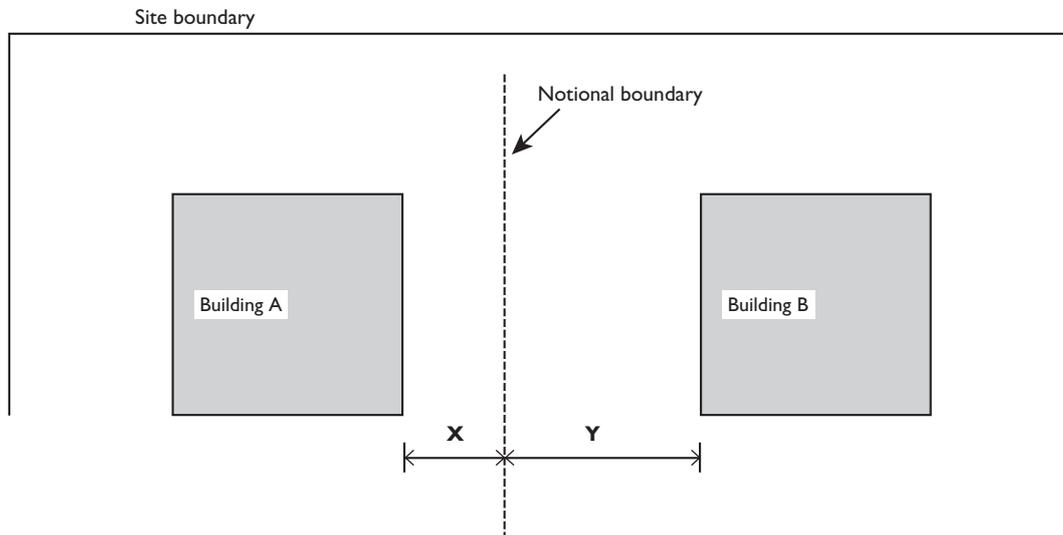
The notional boundary should be set in the area between the two buildings according to the following rules:
