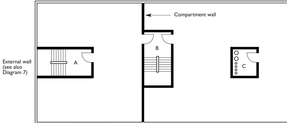
A Protected shaft bounded on three sides by compartment walls and on fourth by an external wall.
