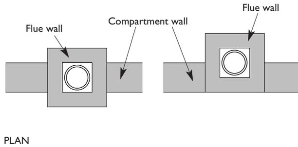
In each case flue walls should have a fire resistance of at least one half of that required for the compartment wall and be of non-combustible construction.
