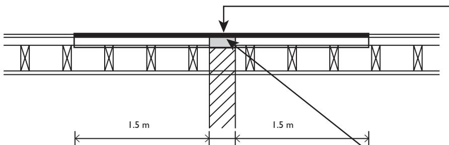
Resilient firestopping to be carried up to underside of roof covering.
