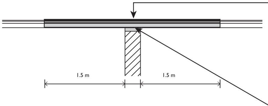
Roof covering to be of class B<sub>ROOF</sub> (τ4) (European class) or to be designated AA, AB or AC (National class) on deck of material of limited combustibility over at least this distance. Roof covering and deck could be composite structure, eg profiled steel cladding.
