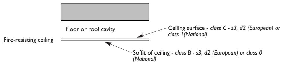
Ceiling surface facing cavity to have surface spread of flame at least class C - s3,d2 (European) or class I (National). Exposed ceiling surface to be class B - s3,d2 (European) or class 0 (National).
