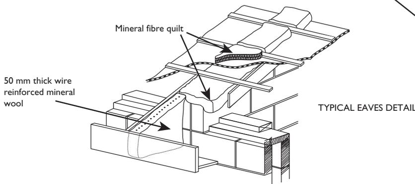
Firestopping to be carried up to underside of roof covering.
